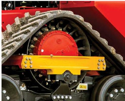
This minimises the impact of power transfer being disrupted while turning and reduces torque loss, making it easier to turn sharply with large implements and heavy loads.
